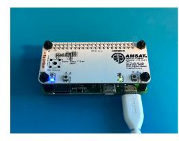
These instructions are for the AMSAT® CubeSatSim Lite vB3. This is a beta release – your comments and feedback are most welcome! The CubeSatSim Lite consists of a Raspberry Pi Zero W (green board on the bottom) with the CubeSatSim Lite board (white board on the top) plugged in with 16 GB micro SD card inserted, secured with nylon standoffs, and a micro USB cable and power plug.
