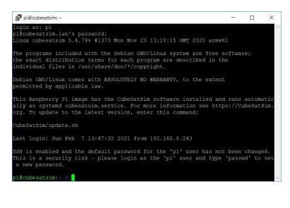
You should set your amateur radio callsign which is transmitted as CW telemetry on 434.9 MHz (+/- 15 kHz) every time the CubeSatSim software starts up. You should edit the CubeSatSim/sim.cfg file to set your own callsign. You can also change localization settings or configure your local WiFi network by running sudo raspi-config.
