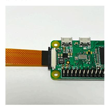
Insert the Pi Zero Camera Cable into the connector. Make sure the metal contacts are facing the PCB, in this photo facing down:
