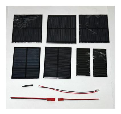
Before using any of your JST connector wires, make sure they have the correct polarity. There is no standard in the industry for red and black, unfortunately, and some suppliers will supply different polarities in different orders. Verify your polarity against this image, and swap if they are reversed:
