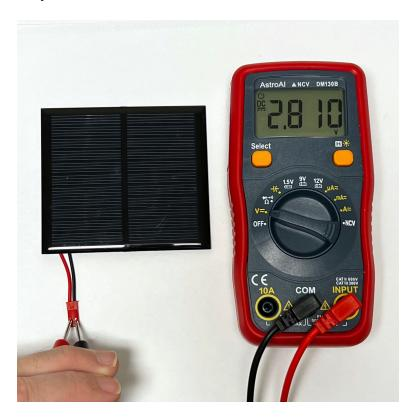
With inside illumination, you should read 1-2 Volts. Outside in the sun or under a lamp, you should read over 4 Volts.
