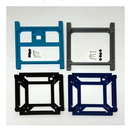
The frame is secured with eight M2.5 x 10mm screws and nuts. If you use a very small amount of hot glue on the edge of the nut well in the frame, you can secure the nut in place - it makes it a lot easier to assemble and disassemble with the nut secured.
