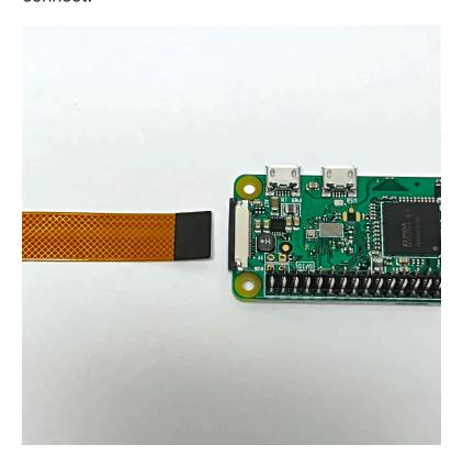
The other end of the Pi Zero Camera Cable connects to the Pi Zero WH on the opposite side to the micro SD card slot. Identify the slide lock, in this photo it is the black plastic:
