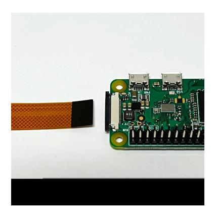
Carefully move the slide lock away from the board, in this photo to the left. Be very very careful - it is very easy to break it. You might need to move it a little on one side, then the other side. It only moves out a few millimeters and does not come completely off. There may be a plastic "blank" in the slot - you can remove it.
