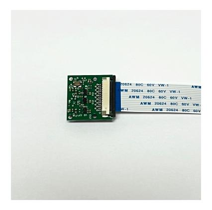
The cable will now be loose and you can slide it out and remove it.
