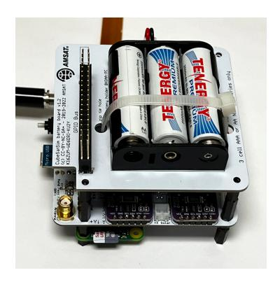
Now create four more of the standoff stacks with the M2.5 15mm+6mm and M2.5 10mm+6mm spacers and insert the threaded end into the holes on the Battery board:
