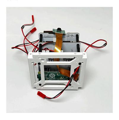
The first frame side to be mounted is the -X side which has the Pi Camera mount. We will mount the frame, the two small solar panels, and also the Camera using Tapered Heat-Set Inserts for Plastic, Brass, M2 x 0.40 mm, and Pan Head Phillips Screws, M2, and two nylon screws and two nylon nuts.:
