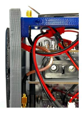
Connect a 90mm x 80mm solar panel to the +Y connector and a 90mm x 80mm solar panel to the -Y connector.
