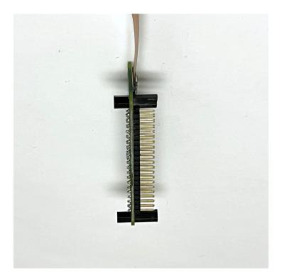
Now, plug the Pi Zero W into the bottom of the Main board.
