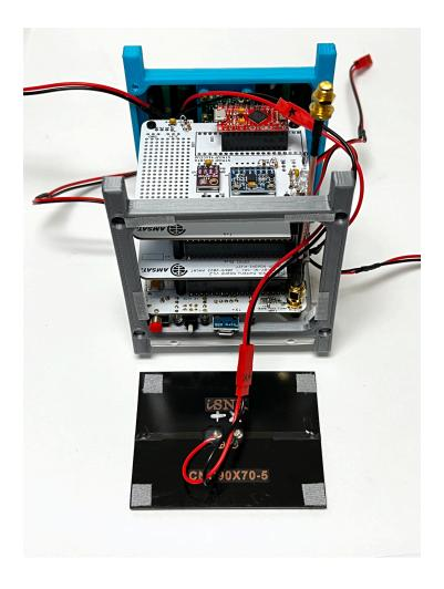
Attach the solar panel to the side frame.
