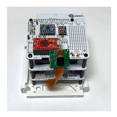
Now, all six JST RCY wires will be mounted on the Main PCB. They should be labeled with the side: +X, -X, +Y, -Y, +Z, or -Z.
