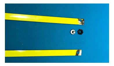
Screw the nut onto the screw, the put the screw through the hole in one of the tape lengths. The screw will cut threads into the center hole of the antenna connector as shown. It can be easier to start the screw in the hole without the tape measure at first to begin cutting the threads.
