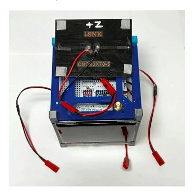
Attach the 90mm x 70mm solar panel to the top frame:
