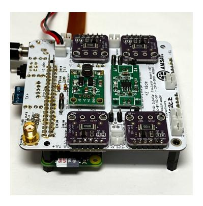
Plug a stacking GPIO header into the board to give the necessary spacing:
