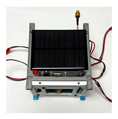
Put the SMA connector through the round hole in the top frame and secure with the nut.
