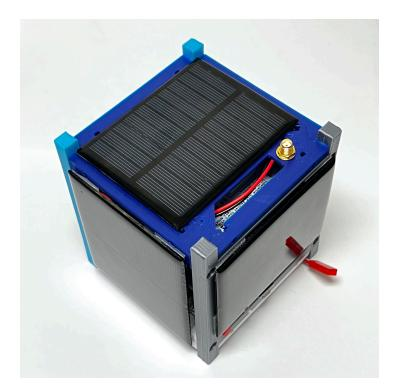
Flip the frame upside down, and connect a 90mm x 80mm solar panel to the -Z connector.
