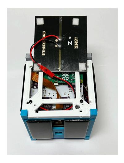
Attach the solar panel to the frame. You will likely need to double up on the double stick tape or foam to clear the screw heads.
