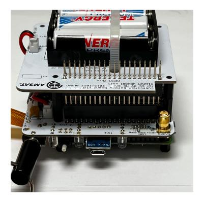
Plug another stacking GPIO header into the Battery board to give the necessary clearance:
