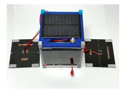
Attach the solar panels to the frame. Note that I'd recommend using velcro to attach these two solar panels and you might need to remove these panels to access connectors or change the micro SD card.
