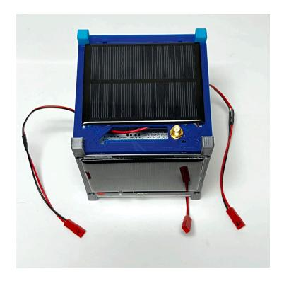
This is the view of the +Y side showing the bend in the SMA coax cable. If your coax is longer than 4", the bend will need to be bigger.
