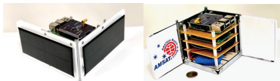
Fig. 8. Figure 8. CubeSat Simulator Winged Frame using Original ETP CubeSat Simulator Sheet Metal Frame.
