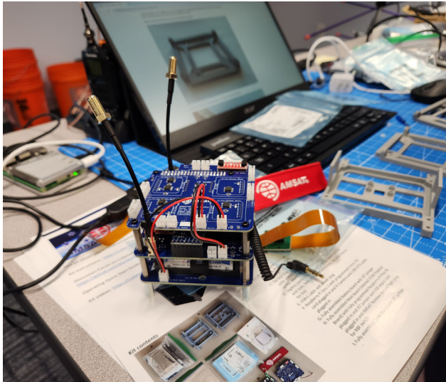
The PCB stack for the no-solder CubeSatSim kit, consisting of a main board, solar board, battery board, and a Raspberry Pi Zero 2 W, assembled during a 2025 ARRL Teachers Institute on Wireless Technology (TI) Space Comms and Radio Astronomy session. [Matt Severin, N8MS, photo]
