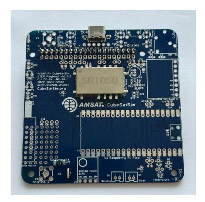
Then solder the 2nd row. The solder should fill the pad but not go up the pin or it will be difficult to insert another board into the connector.
