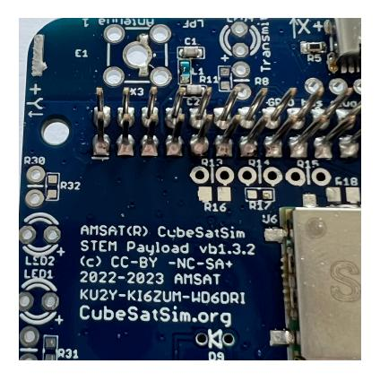
The rest of the components are inserted in the top of the PCB and soldered on the bottom of the PCB.
