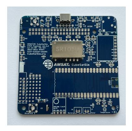
If you aren't good with SMT soldering, you can make a board with just the Low Pass Filters and the FM Transceiver module as SMT, with the USB-C and other components as through-hole soldering. Here are the steps to <u>install the SMT components</u> which will give you this board:
