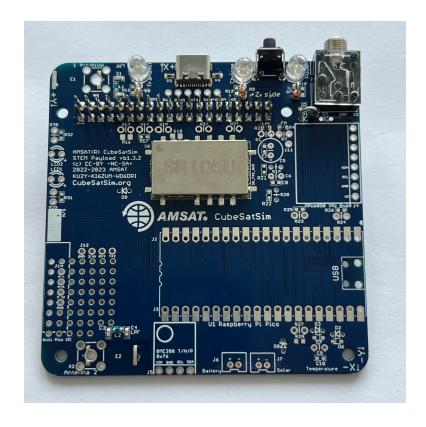
Next install the two 68 Ohm resistors R13 and R15 (big 1/2 Watt resistors with color bands *blue gray black*) and the 180 Ohm resistor R14 (color bands *brown gray brown*) in the attenuator circuit:
