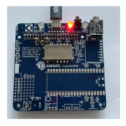
If it doesn't, check LED5, resistor R19, and the USB-C connector.
