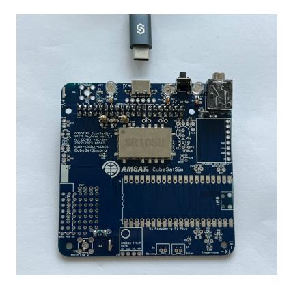
Plug your USB-C cable into a power plug or a computer, then plug it into the USB-C connector on the PCB and the Red LED should illuminate.
