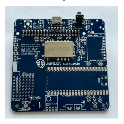
Insert the switch in the top and solder the four leads on the bottom of the PCB:
