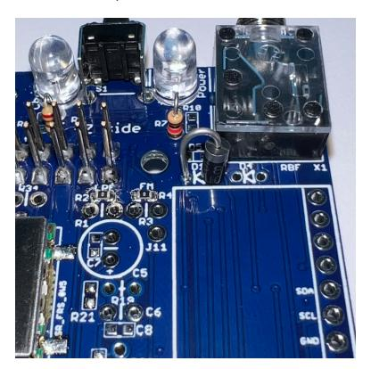
If this diode is backwards, when we plug in the USB-C power cable, the Red LED will illuminate but the board will not power up!
