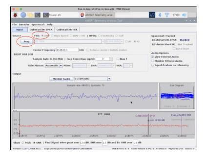
If it doesn't, you might have to click on the FSK DUV radio button or the Start button, circled in red in the image above. This image shows no signal being transmitted by the CubeSatSim. If the CubeSatSim just powered up, it might be transmitting the CW ID, in which case you might see this:
