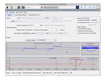
In the FFT window at the bottom of the screen, you can see a peak indicating a transmitted signal from the CubeSatSim, which is circled in red in the above image. Within 30 seconds, if the CubeSatSim is transmitting in FSK mode (mode 2), you should see this:
