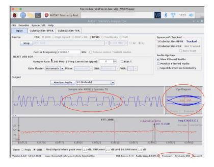
In this image, the digital waveform and the eye diagram are circled in red. At the bottom right of the screen, you should see the Payloads and Frame counts increasing every 4 seconds or so.
