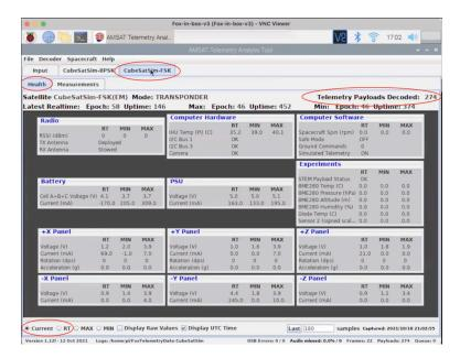
At the top right, the Telemetry Payloads Decoded count should be increasing. If this data isn't changing, make sure the Current radio box at the bottom is selected, indicating that you are seeing live data.
