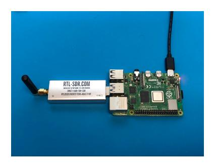
You can write a pre-built Raspberry Pi Ground Station disk image to your SD card. Your Pi 3B or 4B would then boot up immediately running FoxTelem software. This image is based on the ARISS Radio Pi. It has FoxTelem to decode FSK and BPSK telemetry, and also QSSTV to decode SSTV. The Web SDR using OpenWebRX Web will decode the AFSK telemetry by selecting Digital/Packet demodulation.
