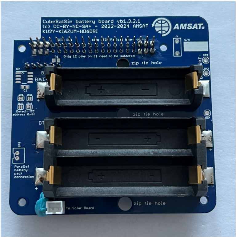
Solder the pins on the other side:
