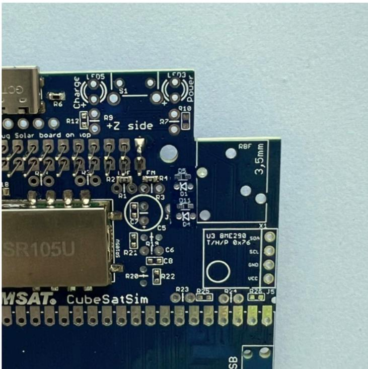
Double check that it is pressed down all the way and straight before going back and soldering any other pins:
