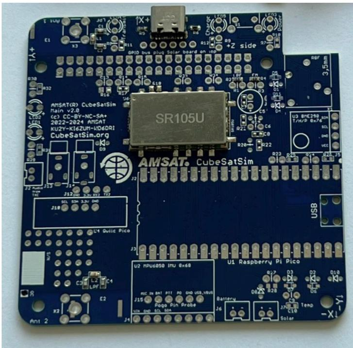
If you aren't good with SMT soldering, you can make a board with just the Low Pass Filters and the FM Transceiver module as SMT, with the USB-C and other components as through-hole soldering. Here are the steps to [install the SMT components](#). (The SMT parts are in the BOM in the SMT Parts tab).
