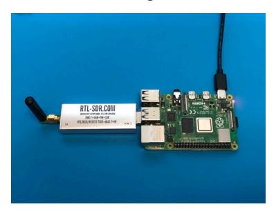
You can write a pre-built Raspberry Pi Ground Station disk image to your SD card. Your Pi 3B or 4B would then boot up immediately running FoxTelem software. This image is based on the ARISS Radio Pi. It has FoxTelem to decode FSK and BPSK telemetry, and also QSSTV to decode SSTV. The Web SDR using OpenWebRX Web will decode the AFSK telemetry by selecting Digital/Packet demodulation.
