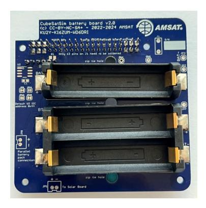
Next, on the top of the PCB, insert the JST connector JP1.
