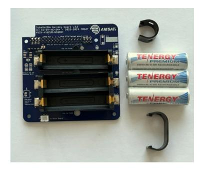
First plug in the batteries, paying attention to the polarity:
