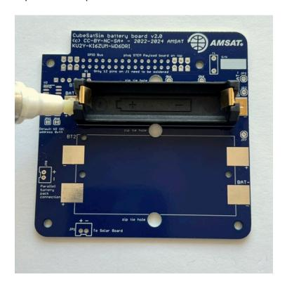
When soldering, make sure you apply some heat to the PCB, not just the part. This will ensure that the solder flows around and under the part
