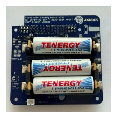
It is a good idea to test your battery polarity using a voltmeter. Use the BAT+ (J1) and BAT- (J2) test points on the board, being very careful not to short them together:
