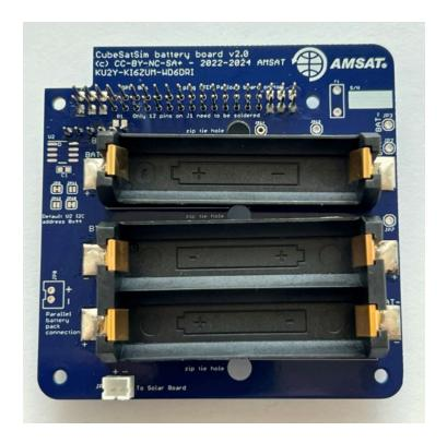
The three NiMH batteries can be inserted and held in place with the clips or zip ties.
