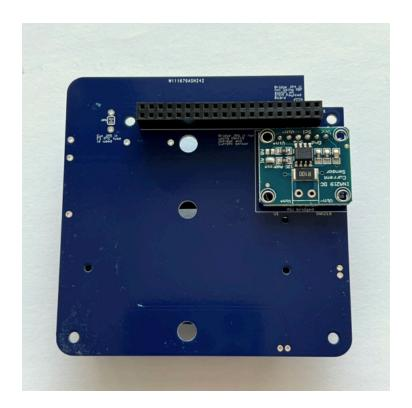
Flip the PCB to the top. Solder one pin on either side, using the pad next to each pin to heat both the pin and the pad:
