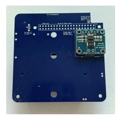
Solder the six pins on top of the INA219 board:
