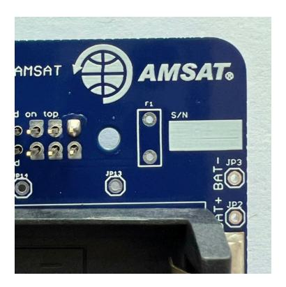
Make sure the GPIO header is fully inserted and straight and on the correct side:
