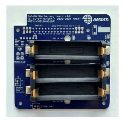
Again, there is a small tab on the bottom of the battery holders that fits in a hole in the PCB - make sure it is inserted so the battery polarity is correct and the holder is flat against the PCB.
