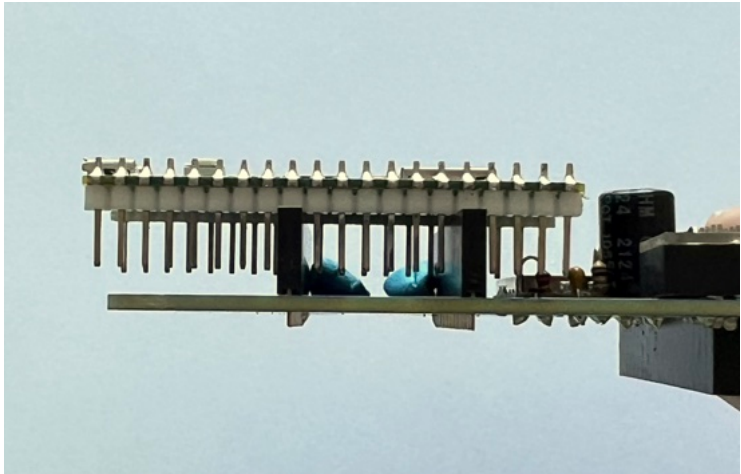
Here is the bottom of the PCB with all the pins soldered:
